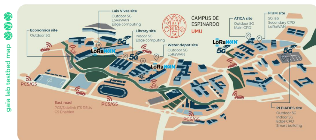
Figure 30: The figure shows the main 5G and edge-enabled sites across the University of Murcia campus, including Luis Vives, ATICA, and Pleiades, interconnected through a private 5G and LoRaWAN network. It highlights outdoor and indoor 5G coverage areas, edge computing zones, and test locations used for vehicular mobility and orchestration experiments.
