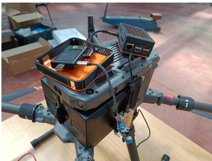
Figure 18: First installation of the USB power consumption meter on the UAV
