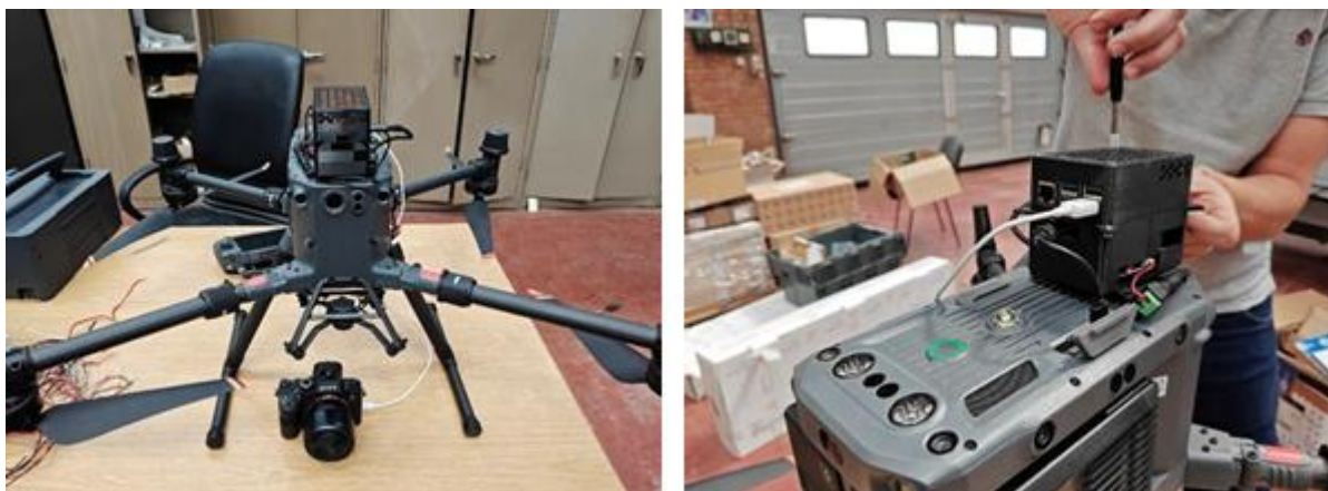
Figure 16: Installation of the Raspberry Pi on the UAV
