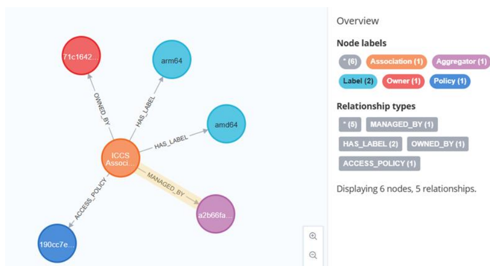
Figure 67: Graph-based representation of the first Association within the Association Metadata Store service.
