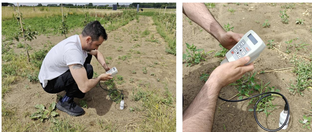
Figure 28: Initial testing of the Delta-T ML3 ThetaProbe soil moisture sensor
