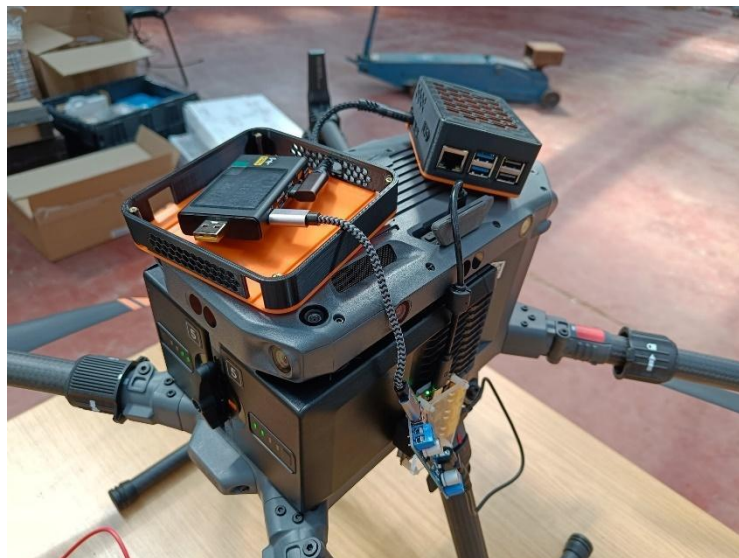
Figure 18: First installation of the USB power consumption meter on the UAV
