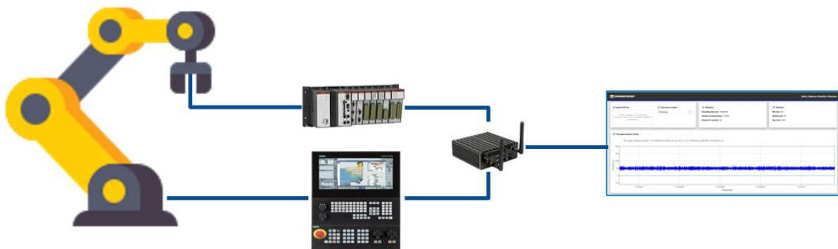
Figure 3: Mid-frequency data acquisition setup integrated into robotic machining systems.
