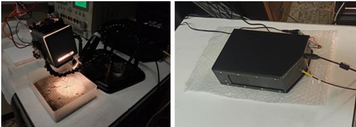
Figure 24: Testing set-up for spectrometer
